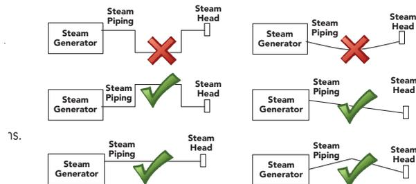
**WARNING** Failure to pitch the steam piping as required for condensate to drain, may cause condensate to block the flow of steam. Blocking the steam flow may cause steam pressure to discharge boiling water through the steamhead, resulting in a scalding hazard. Blocking the flow of steam may cause steam to discharge through the safety valve, resulting in a scalding hazard.
