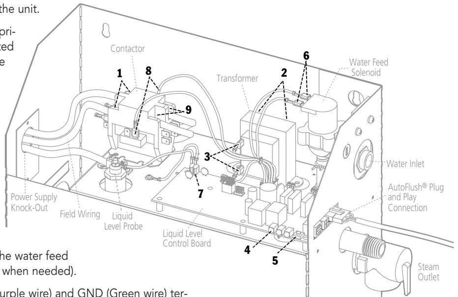
**DO NOT disassemble internal components, internal components contain no serviceable parts.**
