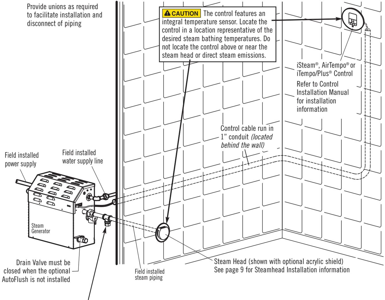
**CAUTION** The control features an integral temperature sensor. Locate the control in a location representative of the desired steam bathing temperatures. Do not locate the control above or near the steam head or direct steam emissions.
