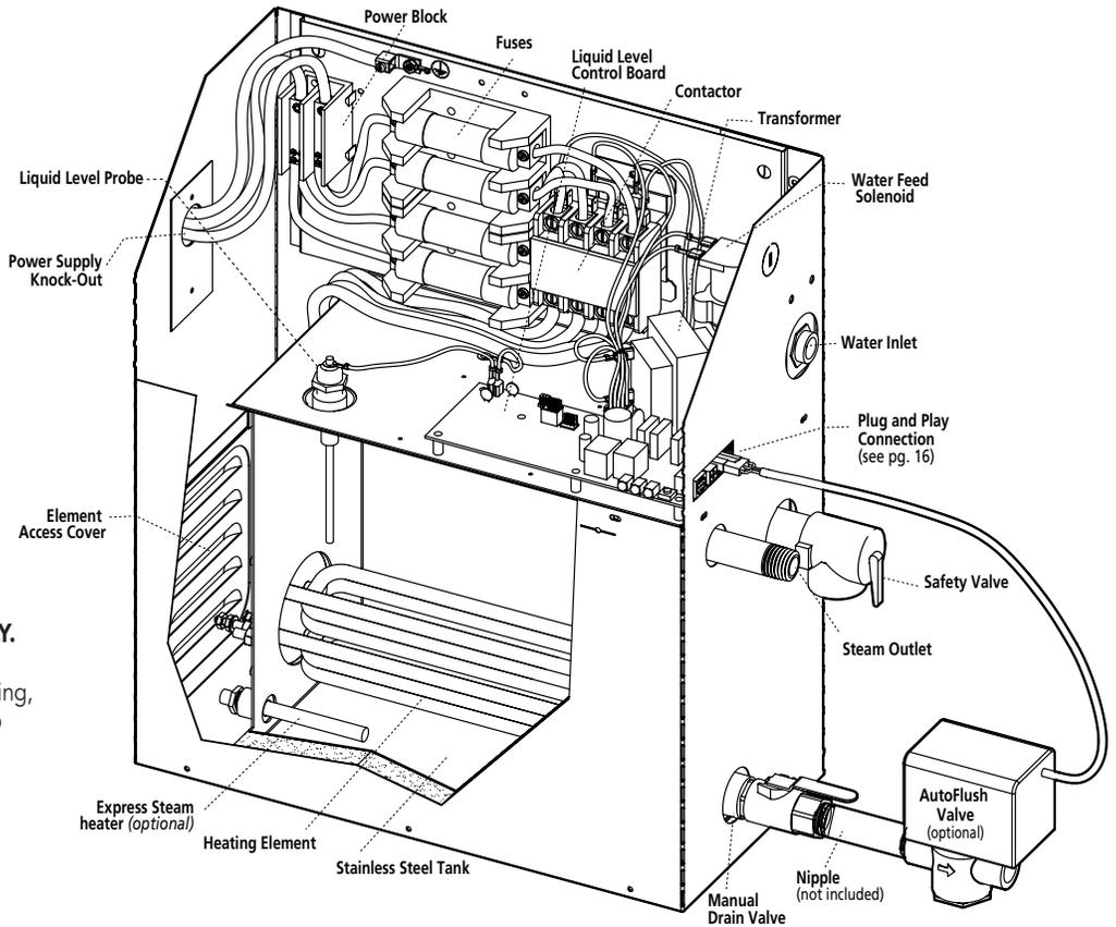
**NOTICE** Super1E 240/1 models are not supplied with internal fusing.
