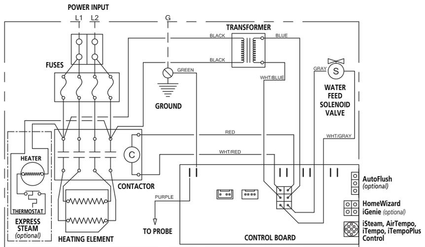
**THREE PHASE 208/240 VOLT WIRING DIAGRAM**
